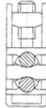
二路电缆连接进线端或出线端 2 nd circuit cable connecting with wire-in or wire-out terminal
